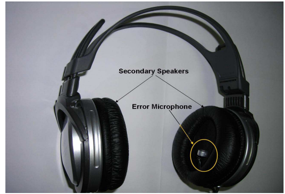
Fig. 4. Basic system configuration
